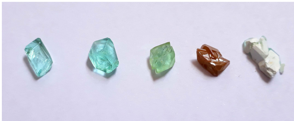
From left to right: 1. Freshly grown crystal; After a month: 2. Sealed in airtight container; 3. Stored in normal container; 4. Left in the open; 5. Stored with a desiccant.
